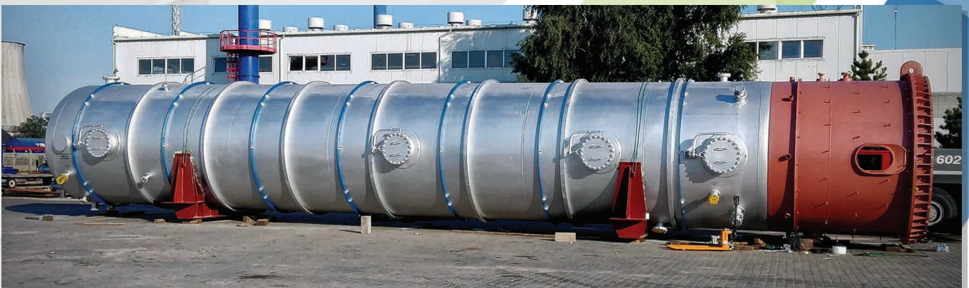
Reactor for bituminous mass system
