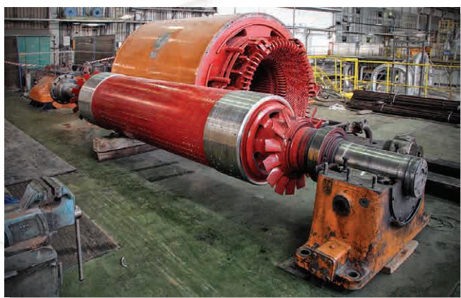
Disassembly of turbine set for Zakłady Azotowe "Puławy" S.A., Poland
