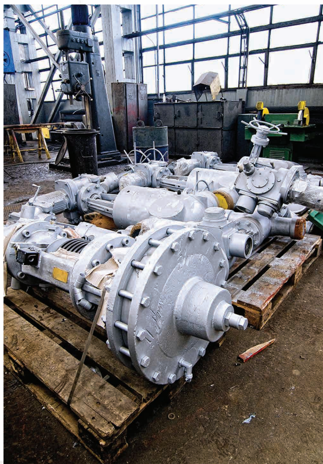
Fitting ready to assembly in steam and system of OP-215 boiler, Poland
