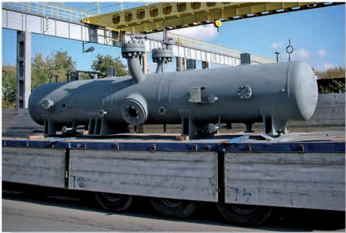
HRS recovery boiler module HRS, type SG-8
