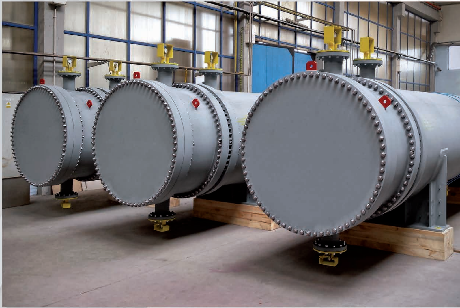
Heat exchanger, type AES – execution acc. to ASME with U-stamp
