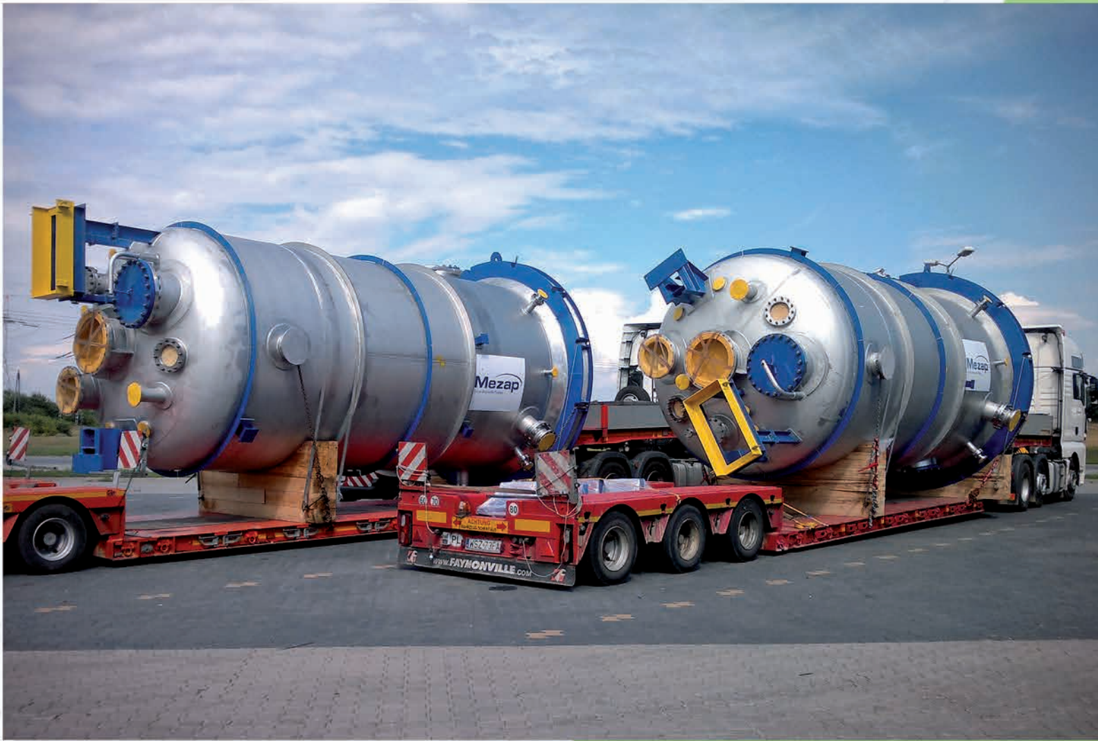
Towers for SSBR project Material grades 1.4462/1.4404.
