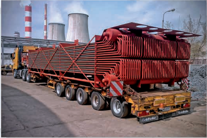
High-pressure preheater PWP-I-TG3
